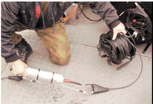
图 10 磁通门传感器定制包装在一个小铝容器中 Fig. 10 Fluxgate sensors tailor-made packaged in a small aluminum container
