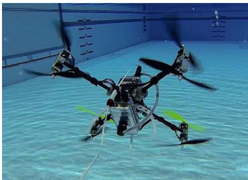
图4 “航海家”潜空航行器 Fig. 4 “Naviator” underwater-aerial vehicle
